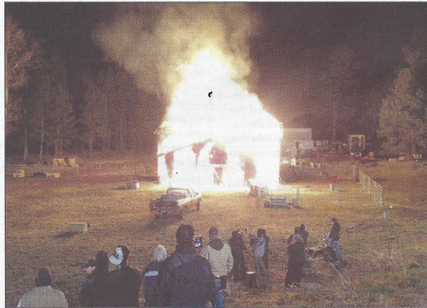
■ A barn on the TV set of A&E’s “Longmire” had to go up in a blaze some 30 times throughout a night of filming. Despite having flames shoot 40 to 60 feet into the air the barn, completely protected by Firetect products, survived the night of burning. Courtesy photo
